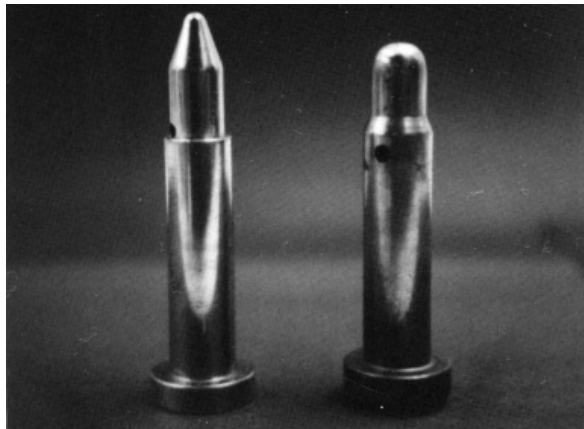
THE CONICAL DART IS PREFERRED FOR MOST INJECTION MOLDED PARTS.
